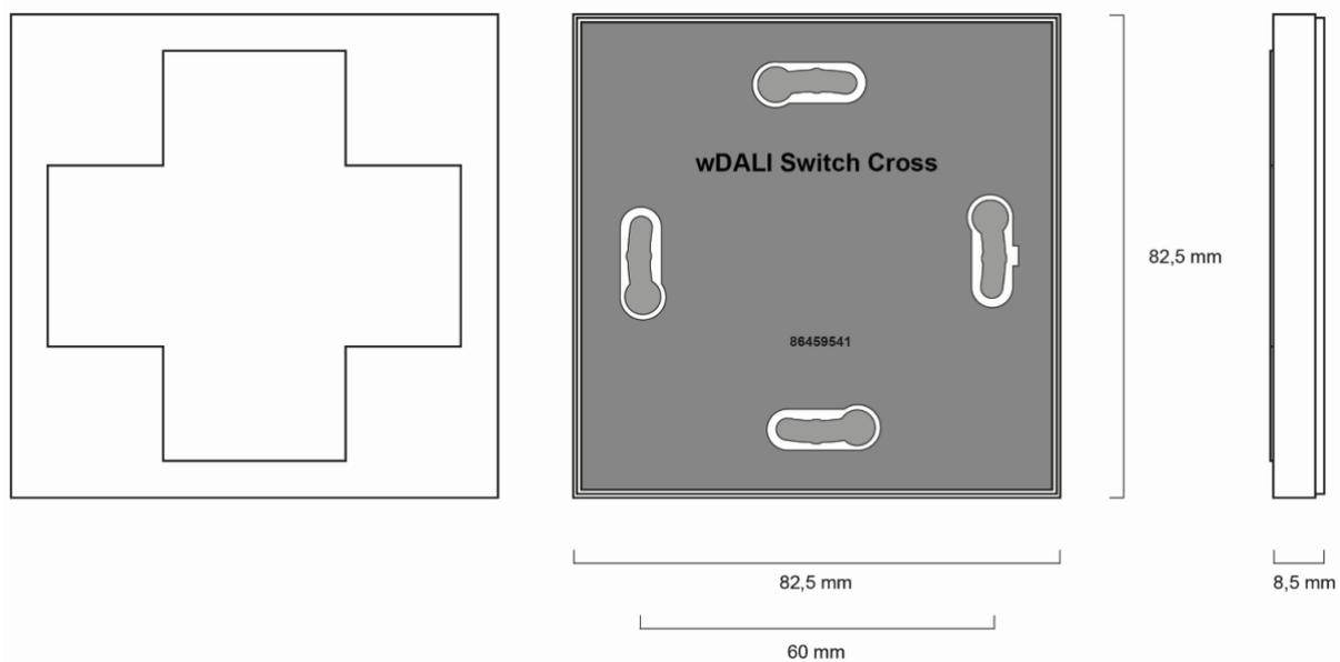
geometry wDALI Switch Cross (input device)
