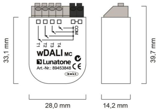
geometry wDALI MC (input device)
