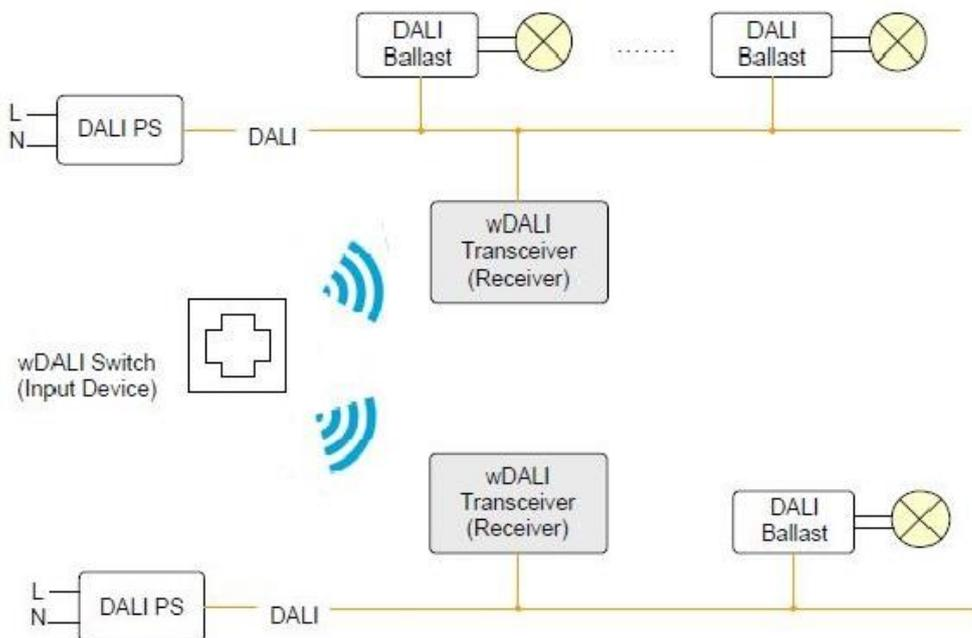
typical installaiton (one input device, simultaneous conrol of multiple DALI-lines)
