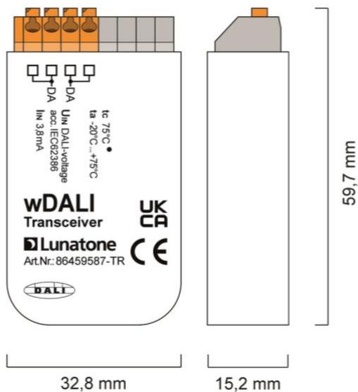
geometry wDALI Transceiver (receiver)
