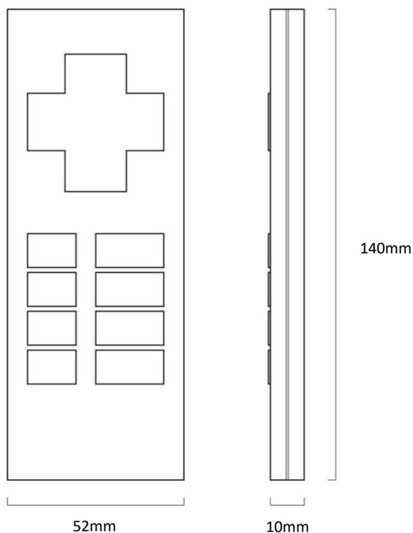
geometry wDALI Remote (input device)
