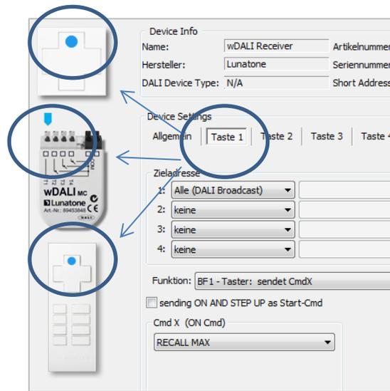
Settings for Switching function of a pushbutton:
