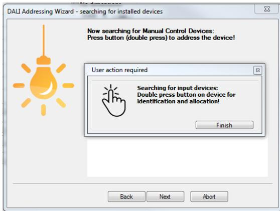
The DALI Touch will be recognized, and an address will be assigned. Afterwards the device can be configured.
