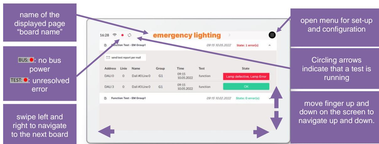
Figure 4 User Interface for Light Control DALI Display 7" Emergency
