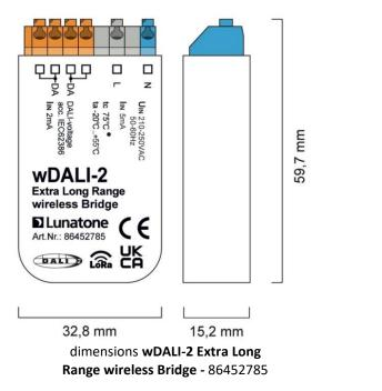
DA DA z lin 2mA **tc** 75°C ● **ta** -20°C ...+55°C DALI-voltage lin 5mA acc. IEC62386 **UIN** 210-250VAC 50-60Hz
