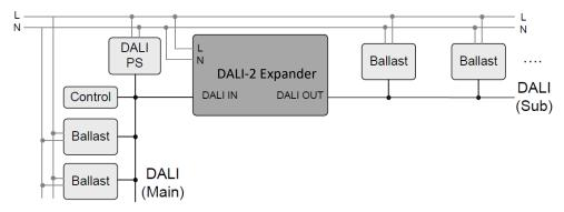
Expansion of a DALI line (Main) with a DALI subordinate line (all control commands sent to the DALI-2 Expander are sent Broadcast to the DALI sub-line.)
