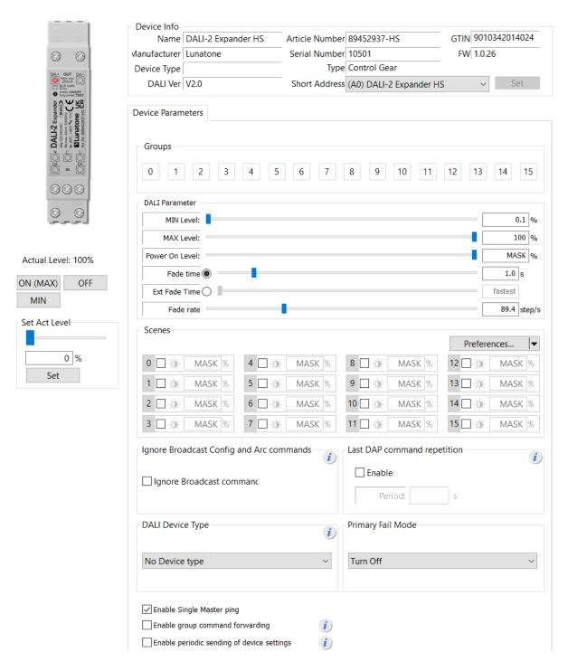
Figure 1 DALI Cockpit Configuration
